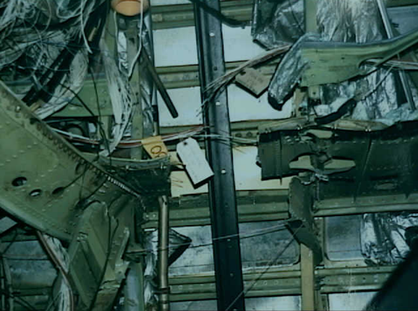
Systems 9 - Fuel Quantity Indication System - Photo 41. W480 (& other) bundles from upper deck at about station 550-590.
