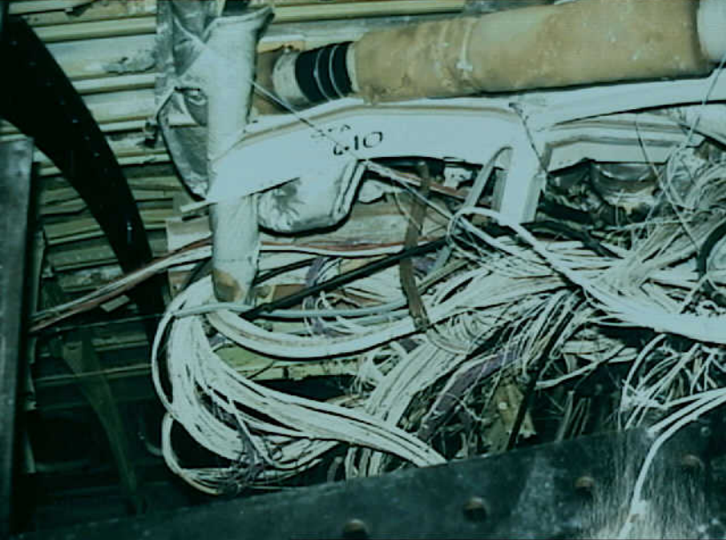
Systems 9 - Fuel Quantity Indication System - Photo 40. W480 (& other) bundles from upper deck at about station 580-630.
