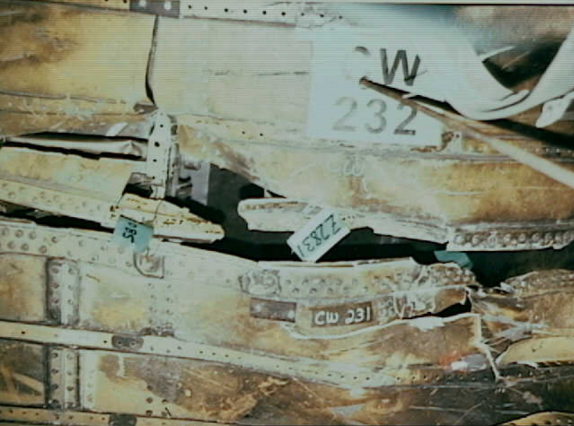
Systems 9 - Fuel Quantity Indication System - Photo 4. Floor of CWT, beneath installed location of compensator. (No negative available)
