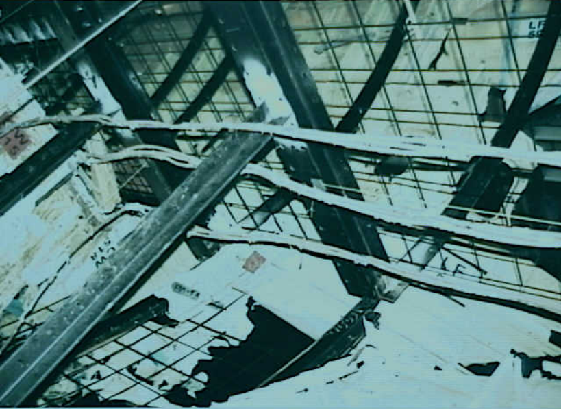
Systems 9 - Fuel Quantity Indication System - Photo 37. Forward spar, breach in left side of fuselage at about station 920 (along route of missing W480 wires), and generator cables for engines 1,2 and APU generator.
