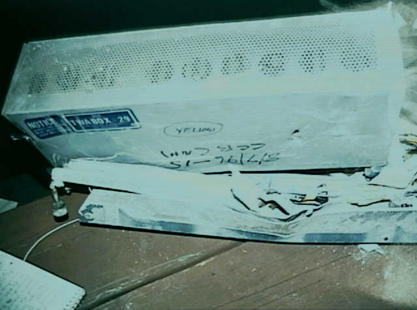
Systems 9 - Fuel Quantity Indication System - Photo 31. AIDS box on E11 avionics rack from upper deck. The features of the adjacent tray and how they align are visible in the scratching near the blue stickers and the puncture that aligns with the (bent) m
