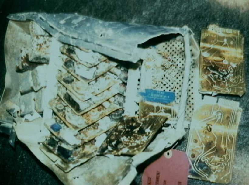
Systems 9 - Fuel Quantity Indication System - Photo 24. Darkened areas on circuit cards in lighting control box from rear of cockpit flight engineer station.
