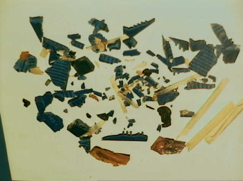
Systems 9 - Fuel Quantity Indication System - Photo 23. Debris from within VSO unit included plastic, metal, and sand. (No negative)
