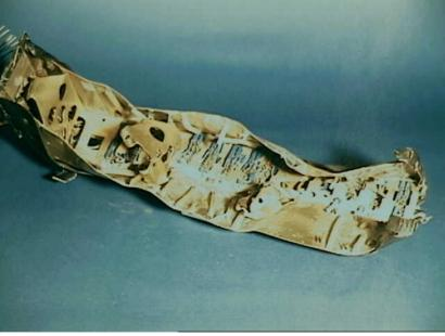
Systems 9 - Fuel Quantity Indication System - Photo 19. Interior of VSO avionics unit after removal of circuit cards. Card connectors (blue) are in the floor of the box. (No negative available)
