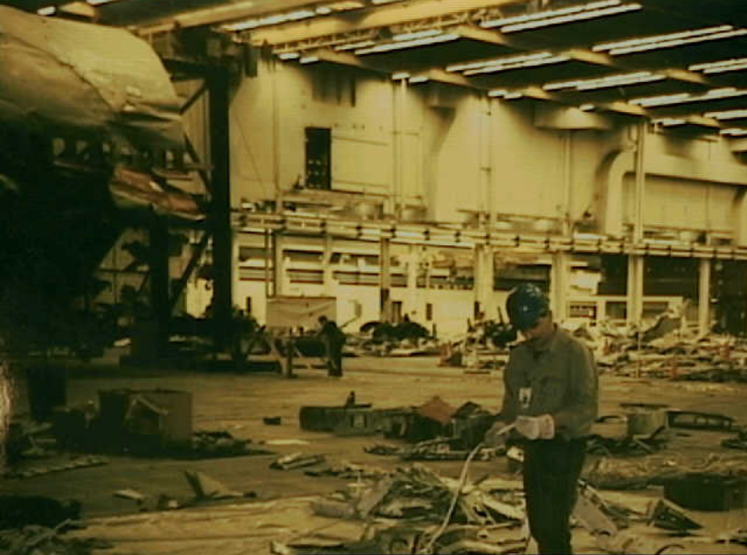
Systems 9 - Fuel Quantity Indication System - Photo 1. Systems group member sorting wires from the forward electronic center (E/E).
