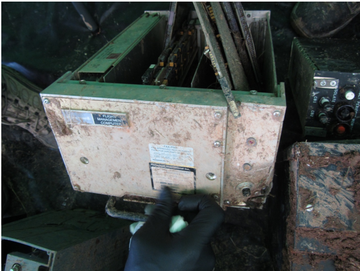
Figure 6 Recovered Flight Management Computer
