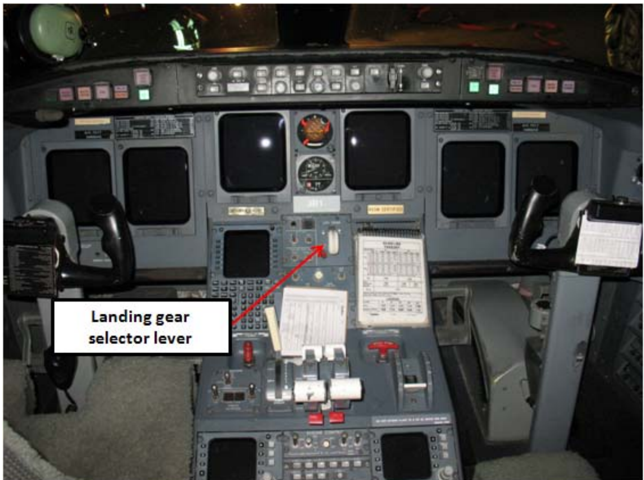
Figure 6 View of the cockpit from an exemplar aircraft showing the landing gear lever
