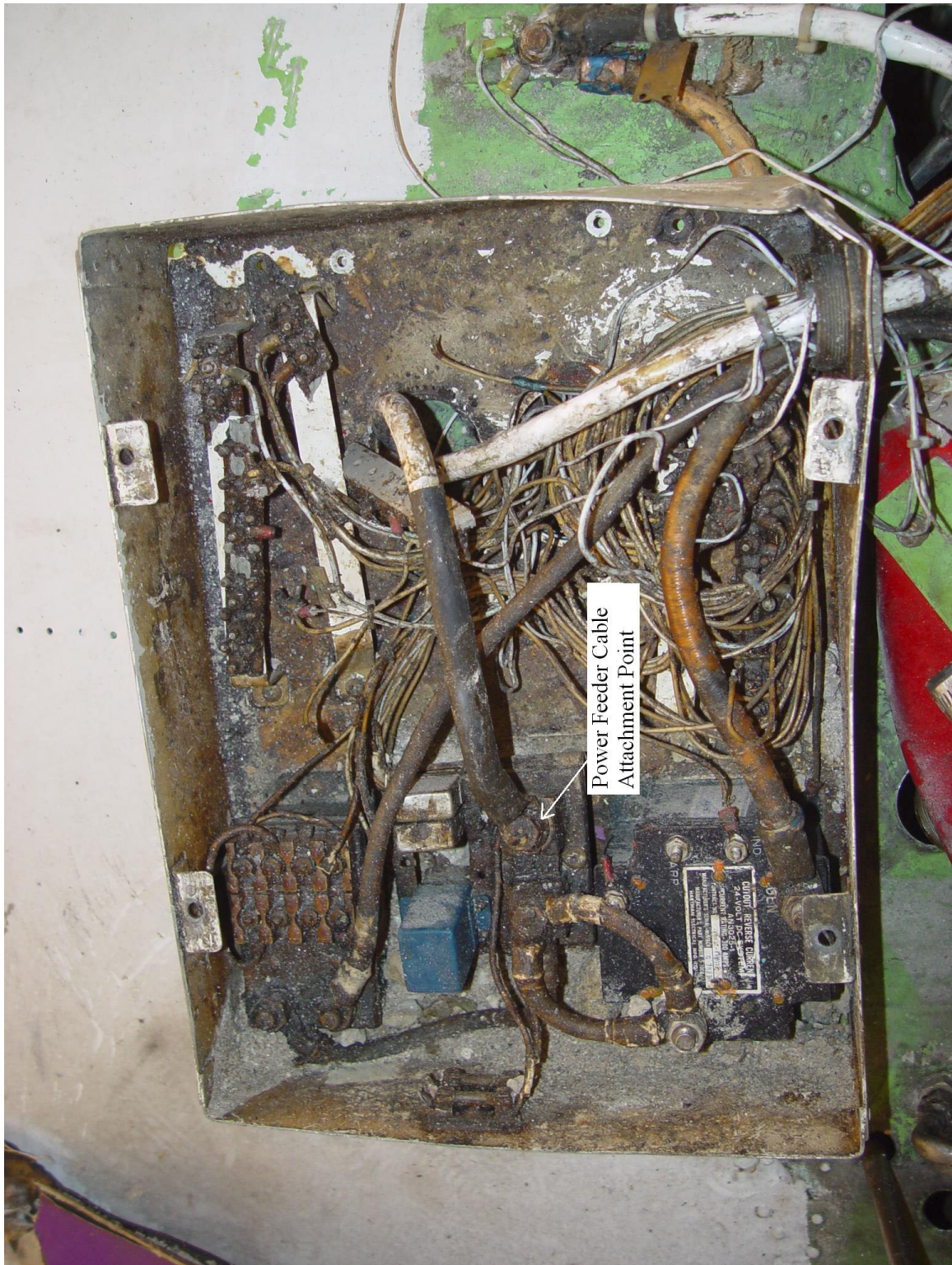
Figure 15. Right wing nacelle junction box.
