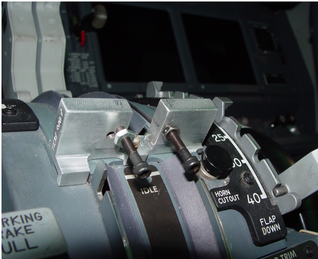
Figure 3 - Tool, shown as installed, used to assist TRA measurement.
