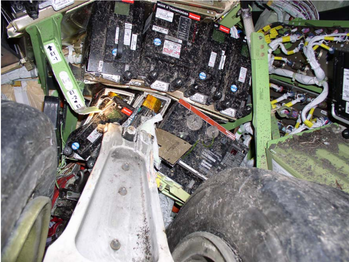
Figure 1 - Damage to Forward EE Bay. Note nosegear assembly.
