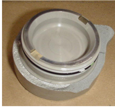
Figure 5 – Fractured Piece of Manifold with End Cap
