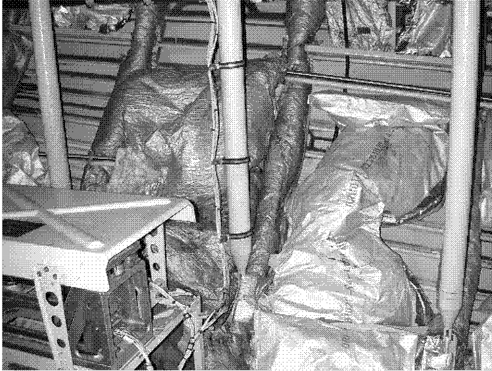
Figure 13 – Close Up View Of Right Side Of Compartment Containing Aft Outflow Valve Showing Displaced Insulation Blankets
