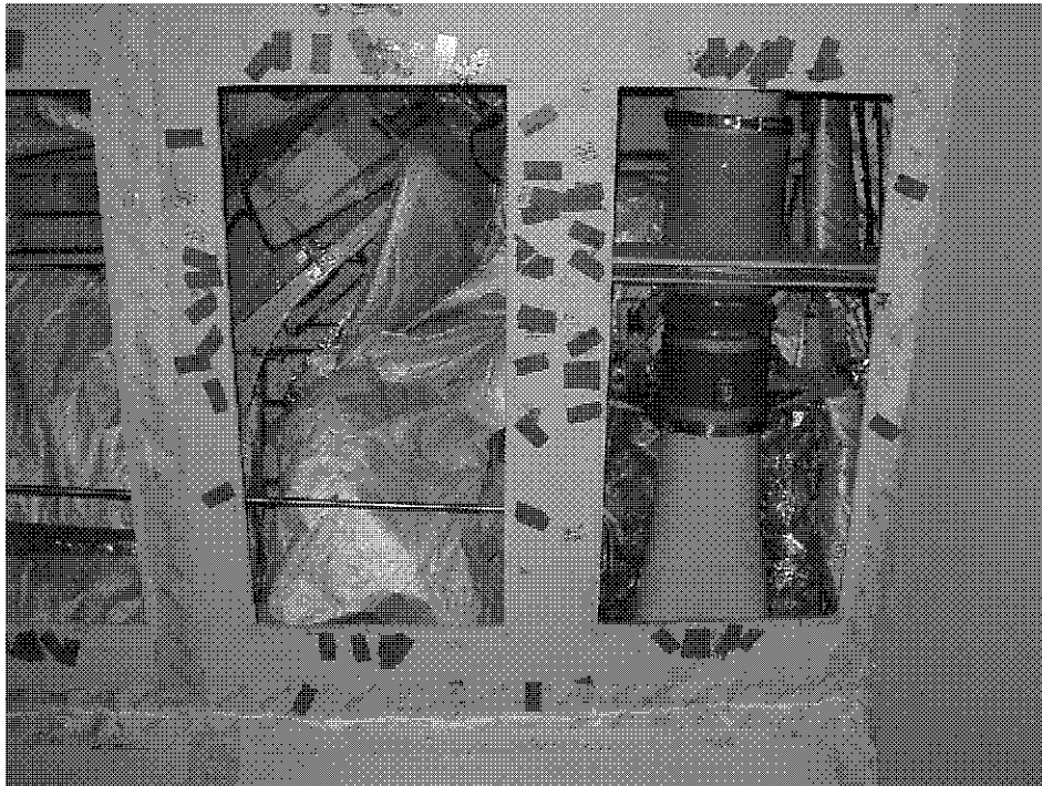
Figure 16 – Right Side Of Compartment (Behind Cargo Compartment Removable Panels) Containing Forward Outflow Valve Showing Displaced Insulation Blankets
