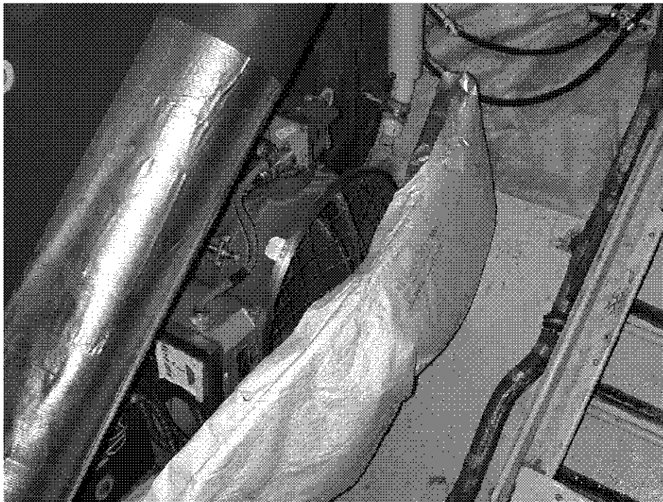
Figure 14 – Forward Outflow Valve With Insulation Valve Partially Obstructing the Intake
