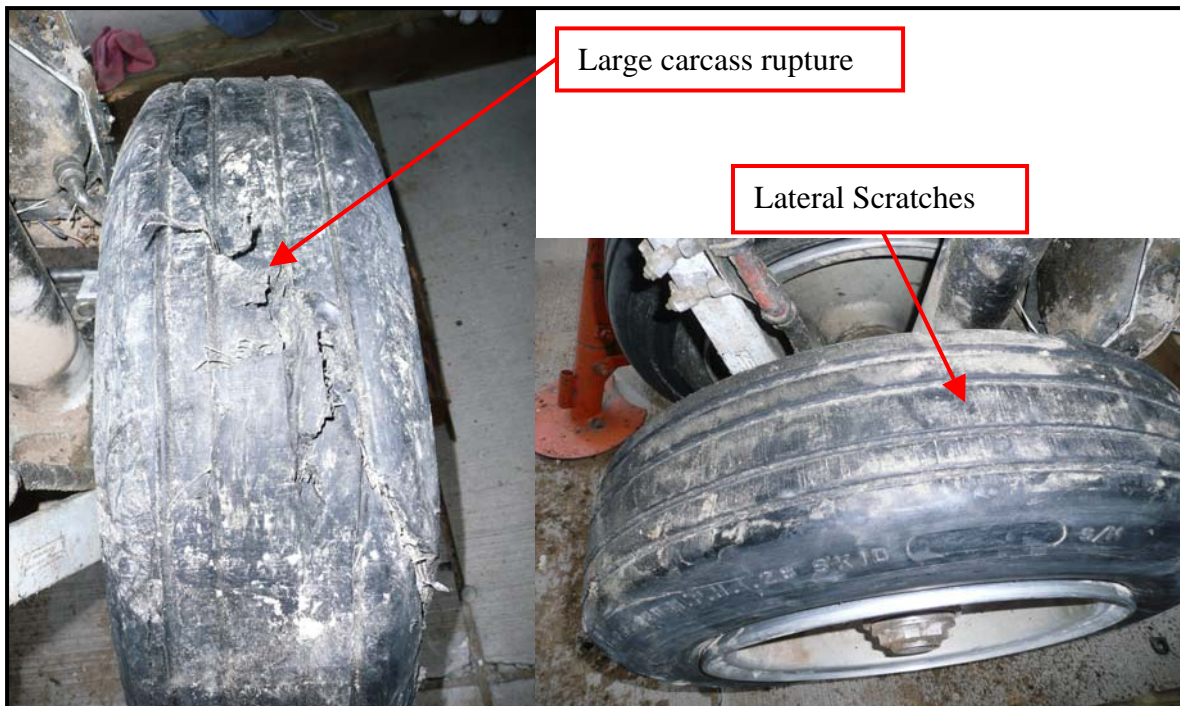
Figure 4 - Photograph of the rupture in the right nose gear tire
