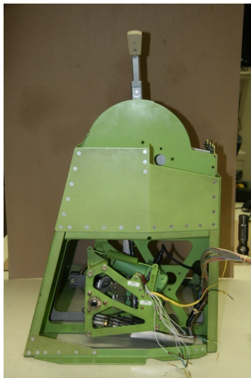
Figure 10 Speedbrake mechanism installed in test stand
