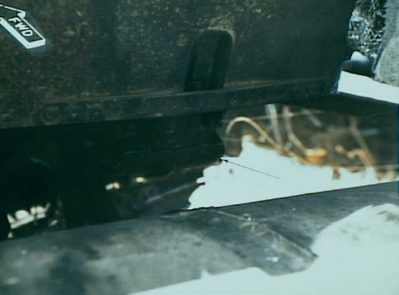
Systems 9 - Exhibit No. 9B - Photo 4. Close-up view (looking forward) of left ground spoiler hinge (arrow). Note extensive heat and soot damage.
