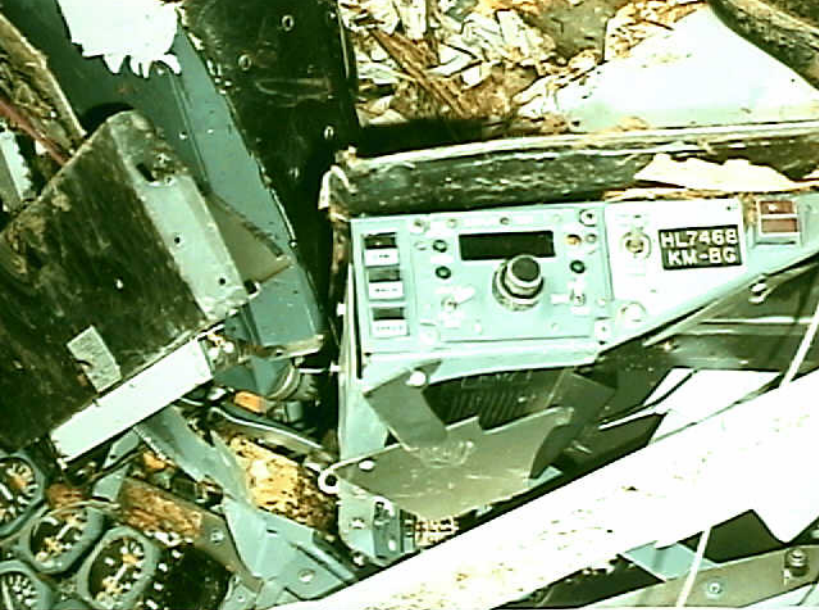
Systems 9 - Exhibit No. 9B - Photo 14. Right Side VHF Control Panel
