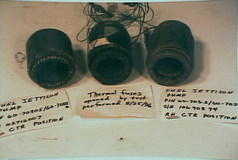
Systems 9 - Exhibit No. 9E - Photo No. 3 - Comparison of motor windings from jettison/override fuel pump from N93119. Center winding was heated until thermal fuses opened and is visibly darker. ATA 28-31-01
