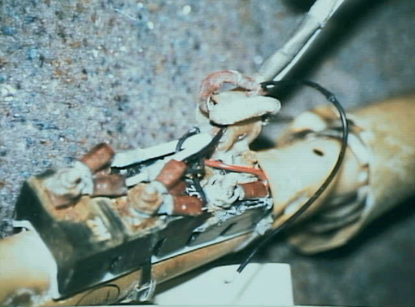
Systems 9 - Exhibit No. 9E - Photo No. 1 - FQIS fragment of #36 with large strain relief clamp (N93119). ATA 28-41-01
