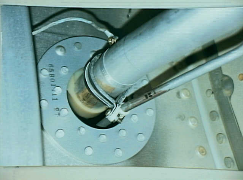
Systems 9 - Exhibit No. 9E - Photo No .4 - Ungrounded Adel clamp on B-747 CWT cross-feed tube (N93105). ATA 28-11-00.
