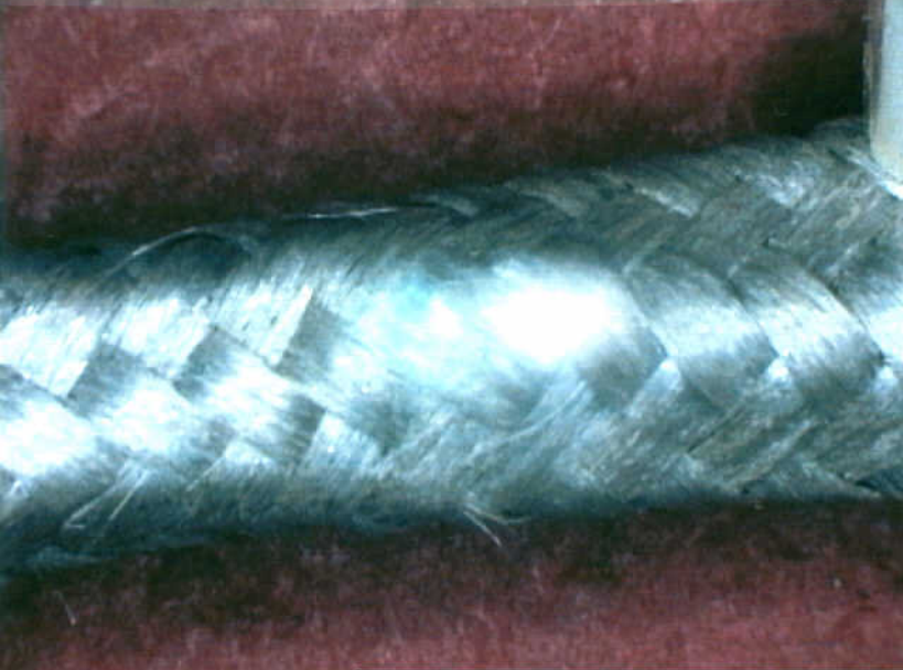
Systems 9 - Exhibit No. 9C - Photo 1 - Splits found in W480 Bundle from N93119 CWT FQIS. Source was external to cut, in routing to cockpit
