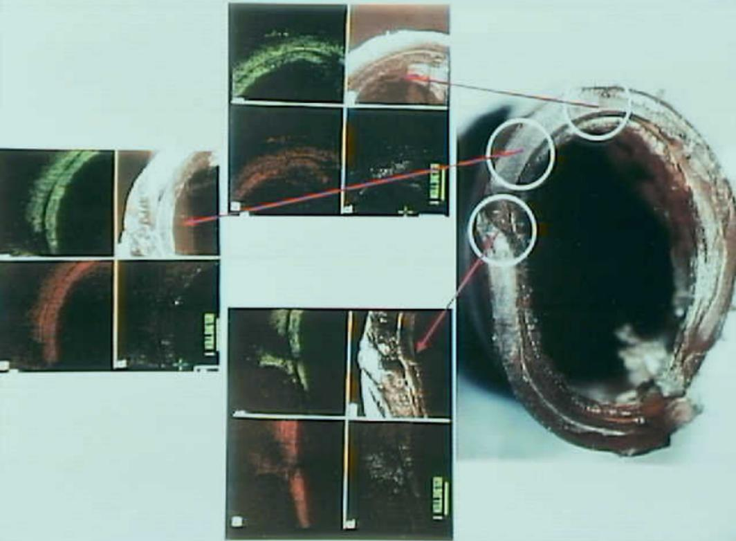
Systems 9 - Exhibit No. 9B - Photo 9. Figure 9g. Insulation surrounding an internal fuel probe terminal. Part was removed from an unidentified fuel probe in the N93110 wreckage. Note darkened regions. X-ray maps of areas were rich in copper and sulfur.
