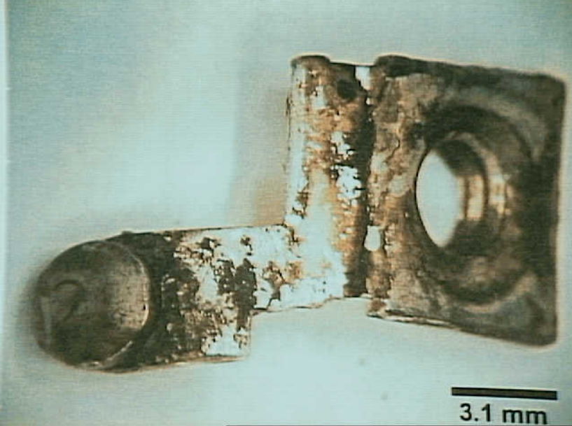
Systems 9 - Exhibit No. 9B - Photo 7. Figure 7c. The stationary line terminal and contact of the SPR circuit breaker have a tarnished appearance.
