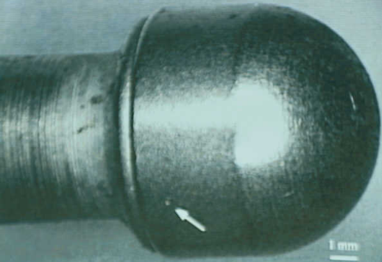
Systems 9 - Exhibit No. 9B - Photo 7. Figure 7a. Gouge found on the left side of the scavenge pump switch knob 15 degrees forward of the knob center line.
