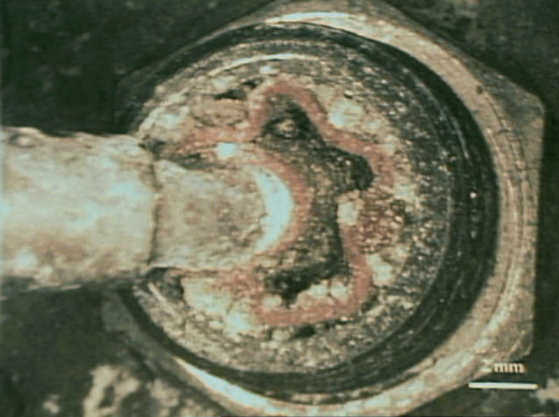
Systems 9 - Exhibit No. 9B - Photo 6. Figure 6a. The environmental seal of the left jettison switch exhibiting corrosion and salt water-like deposits.
