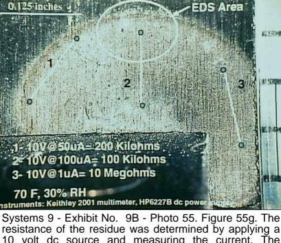
resistance of the residue was determined by applying a 10 volt dc source and measuring the current. The readings were unstable and the above values were maximum current measurements.
