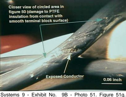
Compensator (model no. FG6C1, serial no. A-166) from N93105 with compression damage to PTFE insulation.
