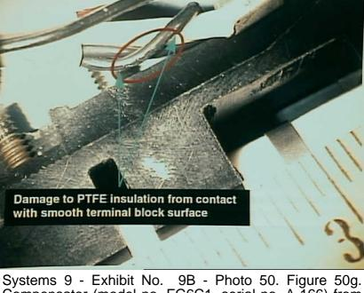
Systems 9 - Exhibit No. 9B - Photo 50. Figure 50g. Compensator (model no. FG6C1, serial no. A-166) from N93105 with compression damage to PTFE insulation.
