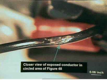
Systems 9 - Exhibit No. 9B - Photo 49. Figure 49g. Fuel probe (model no. FG420A12, serial no. A-9) from N93105 having apparent compression damage to PTFE insulation.
