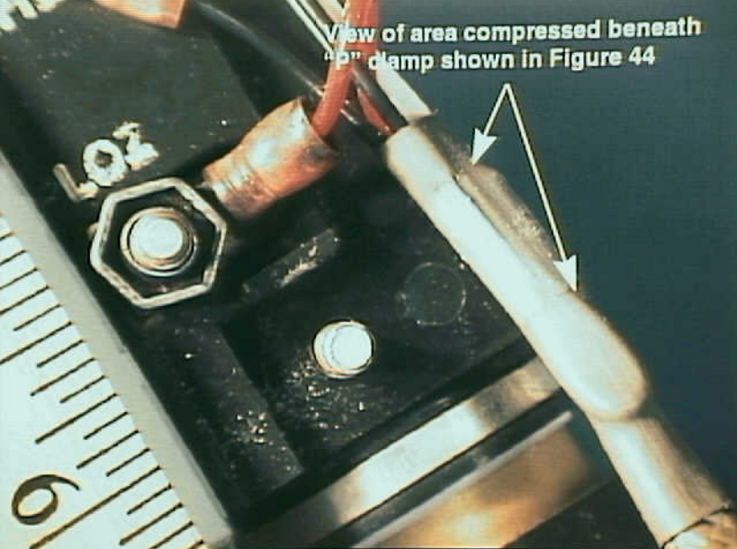
Systems 9 - Exhibit No. 9B - Photo 45. Figure 45g. Wire bundle compressed within "P" strain relief clamp shown in Figure 35 (compensator, model no. FG6C2, serial no. Y-147 from N93105).
