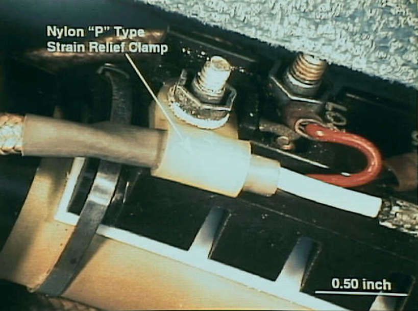
Systems 9 - Exhibit No. 9B - Photo 44. Figure 44g. Example of nylon "P" type strain relief clamp (compensator, model no. FD6C2, serial no. Y-147 from
