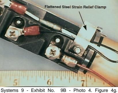
Systems 9 - Exhibit No. 9B - Photo 4. Figure 4g. Termincal block wiring. Wires are dressed differently and the strain relief clamp has been flattened (from N93105).
