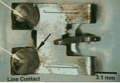
Systems 9 - Exhibit No. 9B - Photo 4. Figure 4c. The moving contacts of the SPR circuit breaker have a tarnished appearance. White arrows highlight the mechanical wear from the making and breaking of the contacts. Black indicates the fibrous residue.
