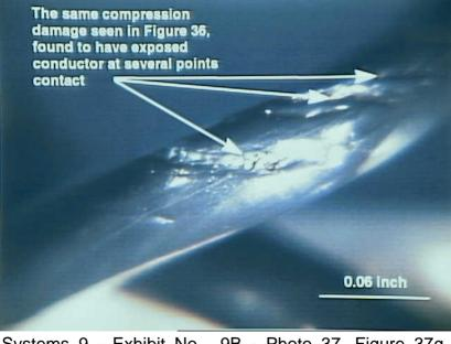
Systems 9 - Exhibit No. 9B - Photo 37. Figure 37g. Compensator (model no. FG6C1, serial no. A-166) from N93105 having apparent compression damage to PTFE insulation.
