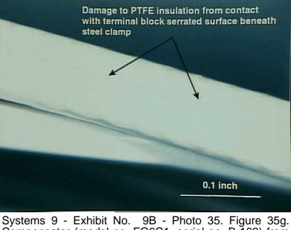
Compensator (model no. FG6C1, serial no. B-162) from N93105 with compression damage to PTFE insulation.
