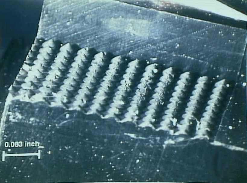
Systems 9 - Exhibit No. 9B - Photo 32. Figure 32g. Closer view of terminal block serrated strain relief clamping surface.
