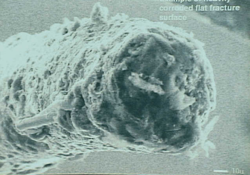
Systems 9 - Exhibit No. 9B - Photo 30. Figure 30g. SEM image--broken shielding wire strand fracture surface.
