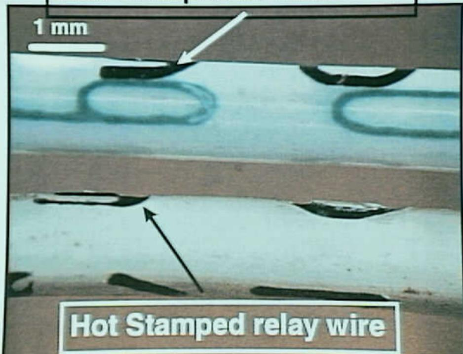
Systems 9 - Exhibit No. 9B - Photo 3. Figure 3f. Note the lack of hot stamp penetration into the insulation of the top wire sample. This was stamped using a current generation machine.
