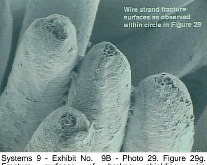
Systems 9 - Exhibit No. 9B - Photo 29. Figure 29g. Fracture surfaces of broken shielding wire strands--necking and dimpling consistent with overload
