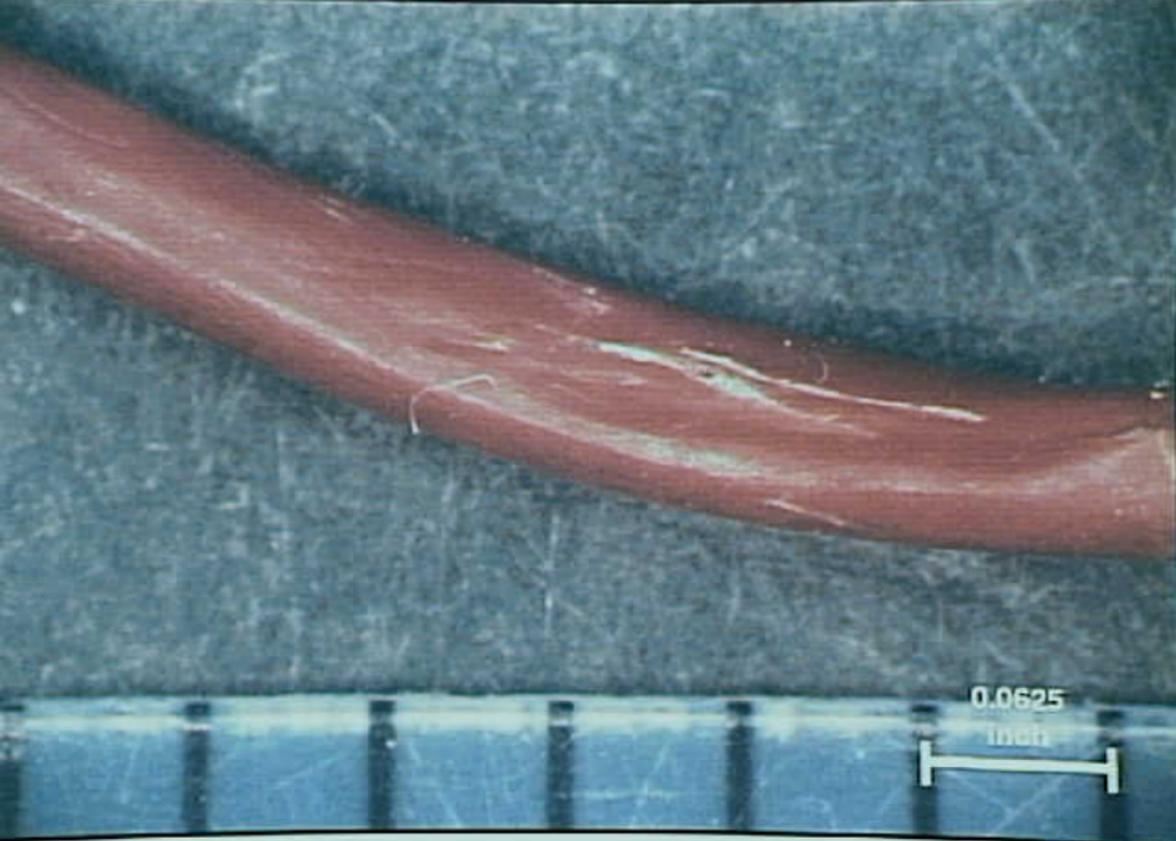
Systems 9 - Exhibit No. 9B - Photo 24. Figure 24g. Compression damage from strain relief clamp (N93119 Fuel probe sample #5).
