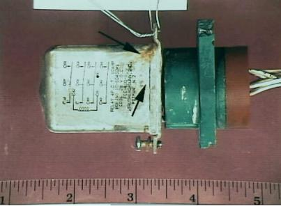
Systems 9 - Exhibit No. 9B - Photo 2. Figure 2b. Scavenge pump relay. Arrows show the reddish brown and white residues on the case of the relay.
