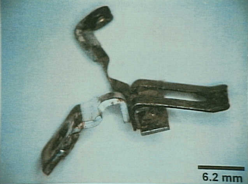
Systems 9 - Exhibit No. 9B - Photo 18. Figure 18c. The stationary load terminal and contact of the RTV circuit breaker have a tarnished appearance.
