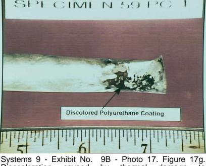
Discooloration caused by thermal damage polyurethane coating (from N93119).
