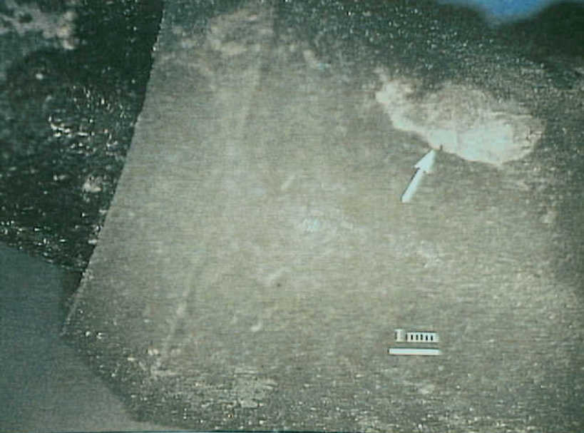
Systems 9 - Exhibit No. 9B - Photo 17. Figure 17a. Right jettison switch plunger guide exhibiting typical mold runner marks (arrow).
