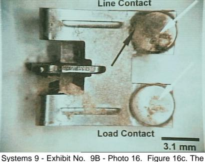
Systems 9 - Exhibit No. 9B - Photo 16. Figure 16c. The moving contacts of the RTV circuit breaker have a tarnished appearance. White arrows highlights mechanical wear from the making and breaking of the contacts. Black arrow indicates fibrous residue.
