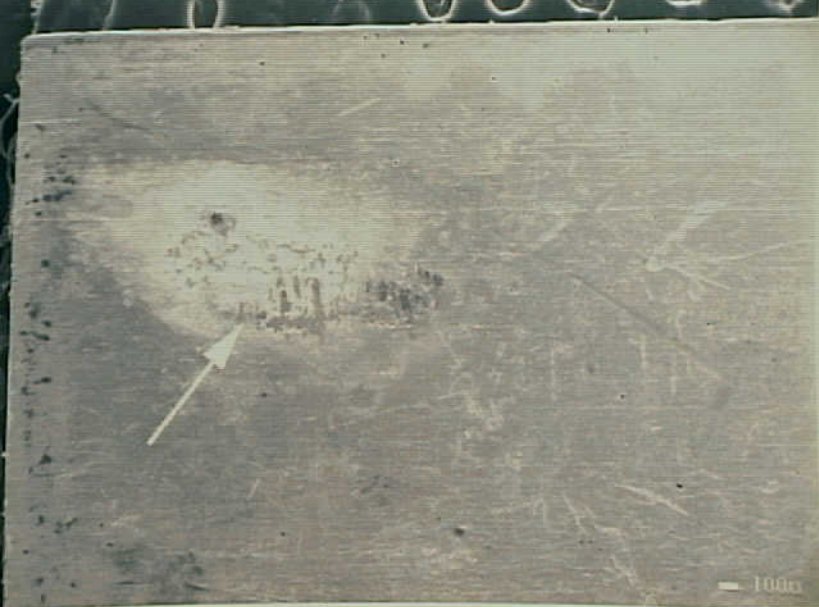
Systems 9 - Exhibit No. 9B - Photo 15. Figure 15b. Mating surface of moving contact A2. Arrow shows the contact area.
