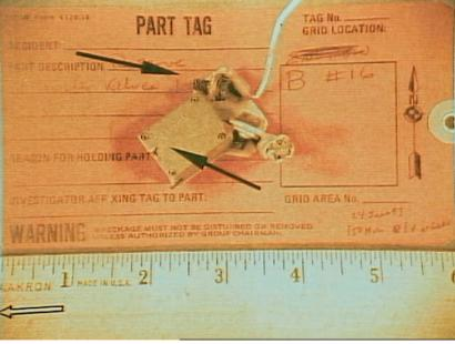
Systems 9 - Exhibit No. 9B - Photo 14. Figure 14c. As received condition of the RTV circuit breaker. Upper arrow highlights the corroded terminal harware. Lower arrow highlights the cracked housing.
