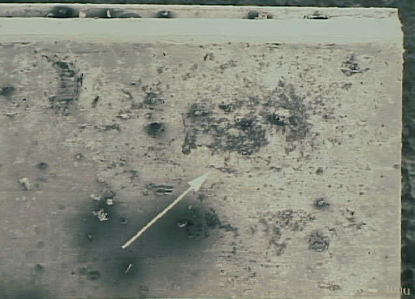
Systems 9 - Exhibit No. 9B - Photo 14. Figure 14b. Mating surface of stationary contact A1. Arrow shows the residue covering the contact area.
